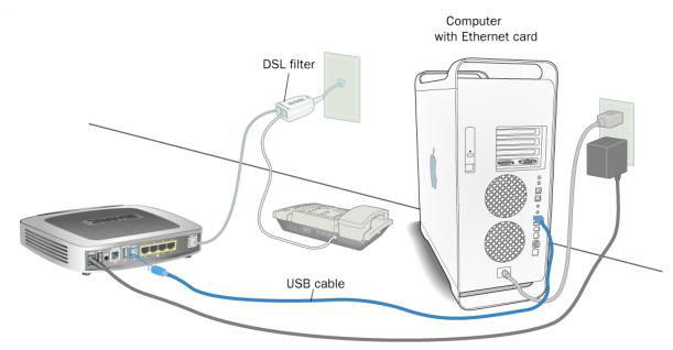
Figure 8. Gateway Connected Via USB (Macintosh)
